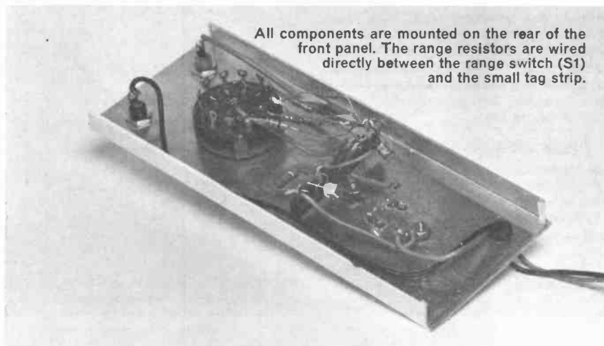
Fig. 2. Layout of components, interwiring and front panel details. Note that S1 consists of one section of a 2 pole-6 way rotary switch with two positions unused.
