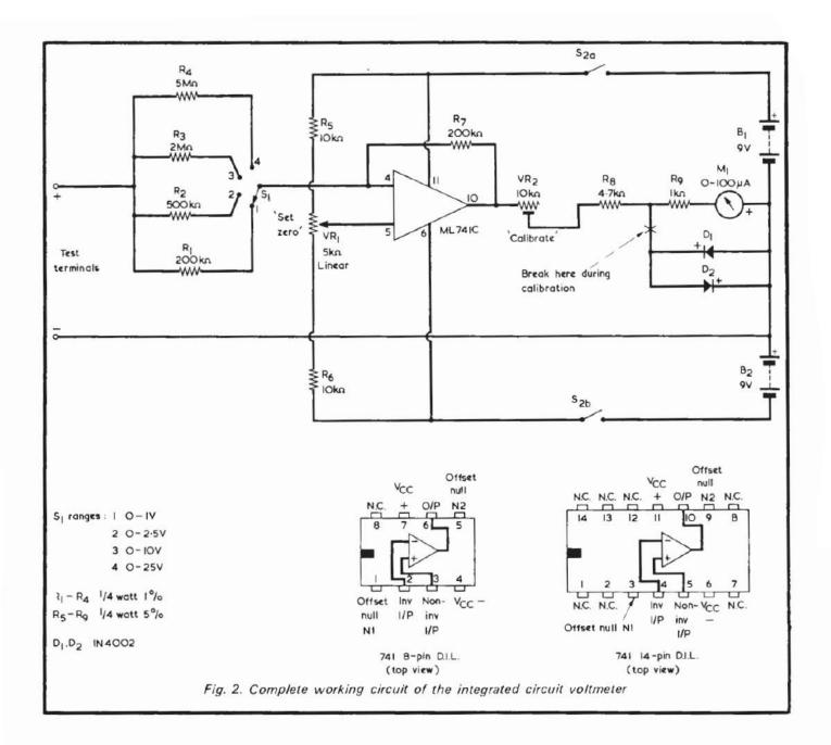
range would be  $600k\Omega$ . Any other ranges within reason can be incorporated by employing the appropriate multiplying factor for the series resistance required. In this version of the input switching circuit the series resistors should all have a tolerance of 1%.
