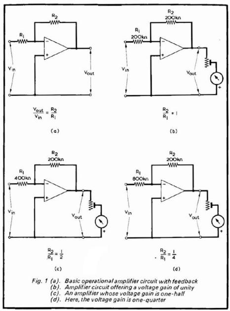
we apply a voltage of I volt to the input, the output will also be I volt, and the meter will read full-scale deflection. The polarity of the input voltage is such that the upper input point is positive. Since this point is coupled to the inverting input of the op-amp, the op-amp output will be negative. This output polarity corresponds with the polarity ascribed to
