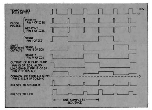
Need an adjustable waveform generator? The Rhythm and Blues Box can handle that too. Simply tap in at the appropriate point, hook up your scope, and you're ready to go.
