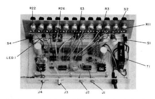
With the cover removed, the placement of all components can be observed. When wiring the front panel pots, it's a good idea to tag the wires from the PC board for identification. For more work room, install only every other pot at first, wire, then install the rest.
