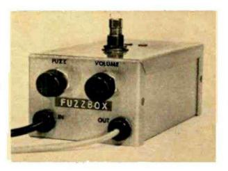
Our model has cables which plug into your guitar and amplifier. Step on push-button switch on top and you add fuzz; step again and you remove it.
